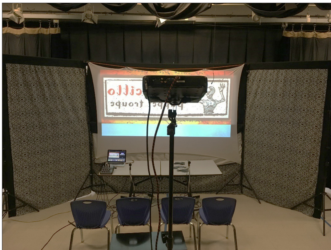
Figure 1: A backstage view of the shadow puppet stage configuration, illustrating the projector situated behind the performers, the screen displaying the image in reverse, and the laptop, sound mixer, and microphones used to control the audio-visual elements of the performance. 3
